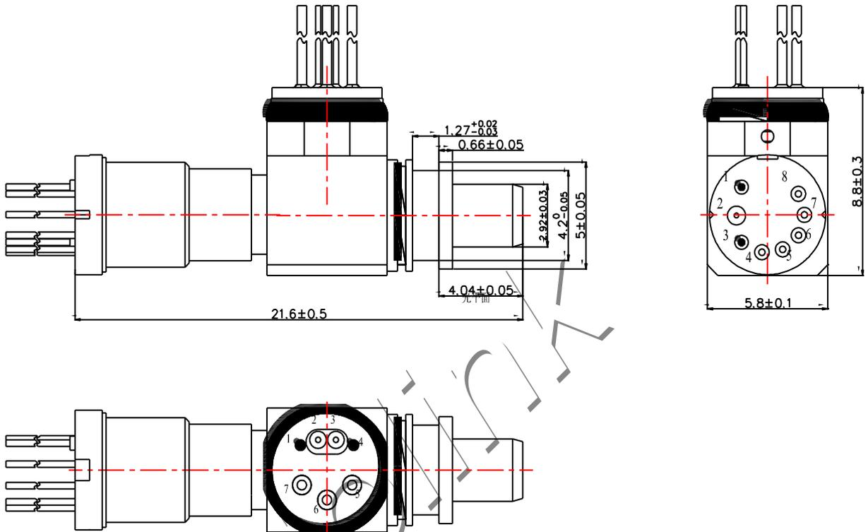
Note2: PIN direction and laser mark can be customized.
